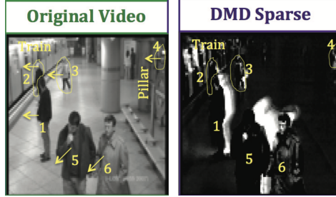
Figure 1: On the image on the right, only high frequency modes are reconstructed (i.e: taken into account in the sum in (2.13)), leading to an effective removal of the static ( \omega_k \approx 0 ) background. (Image adapted from [12])
