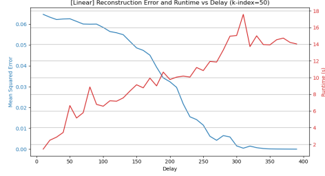
Figure 28: Error and processing time as a function of the delay introduced in Hankel pre-processing.
